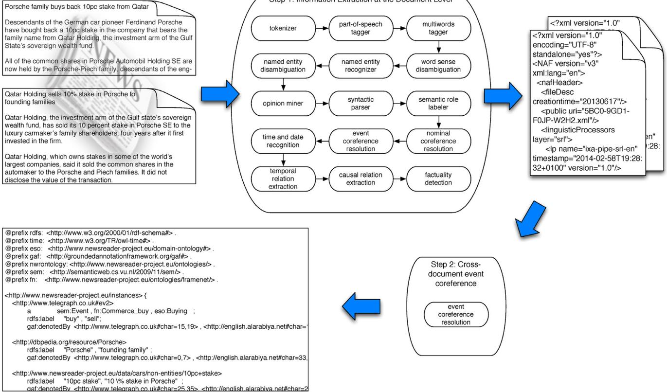
Fig. 1. Overview of the NewsReader system taking raw text as input, creating XML representations (NAF) for NLP output and creating RDF representations (SEM) from the XML representations.
